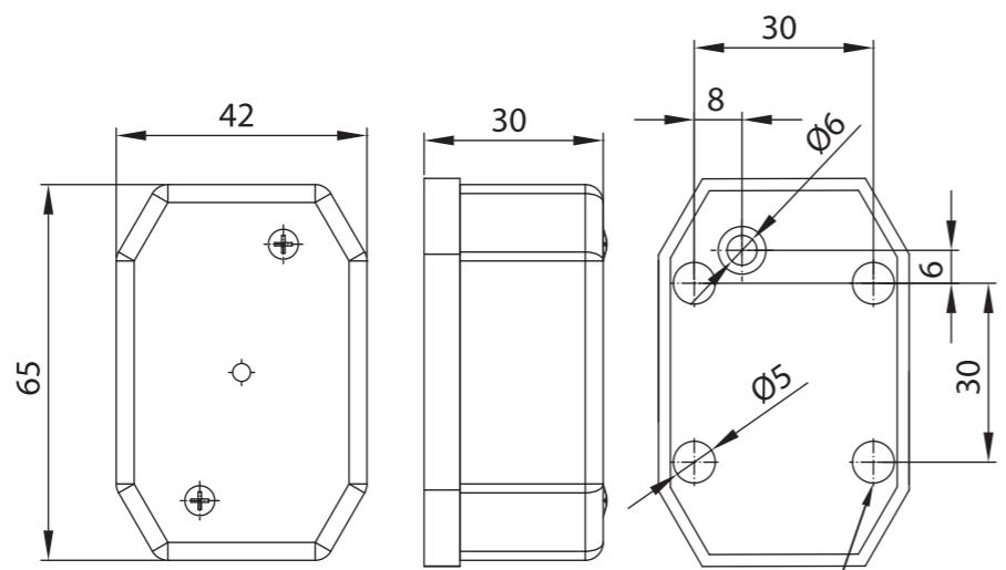
mounting openings for a metal-sheet screw
