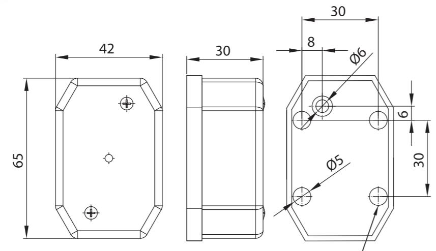
mounting openings for a metal-sheet screw
