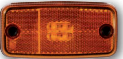
1-functional LED clearance lamp with a reflector
