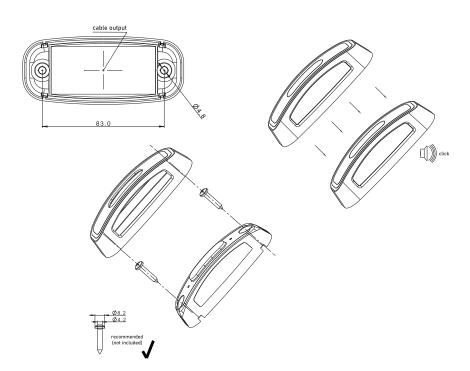
LED clearance lamp, tree-functional, with a sidelight (front, tail and side), 0.5 m long cable.
